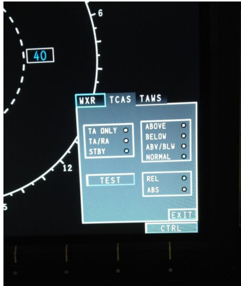
Figure 4-5 MFD TCAS II controls when CTRL button key (B-8) is pressed on the MFD (Sheet 1 of 2)
