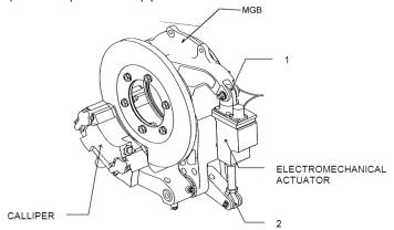
Secure the calliper in the down position connecting the bolt holes (1) and (2) with a tie-wrap strap. Secure the free connector of the actuator using a tie-wrap strap. Pull the PWR and the CONTR circuit breakers on the RTR BRK section of the overhead circuit breaker panel. Secure the system by locking all the deactivated circuit breakers and tag accordingly.
