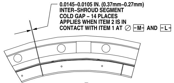
VIEW P SHOWING ONLY SHROUD HOUSING AND SHROUD SEGMENT LOOKING DOWNSTREAM
