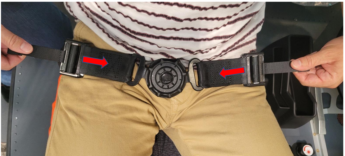
PHOTO 4 - Action of pulling the adjustment tabs of the lap straps towards the buckle
