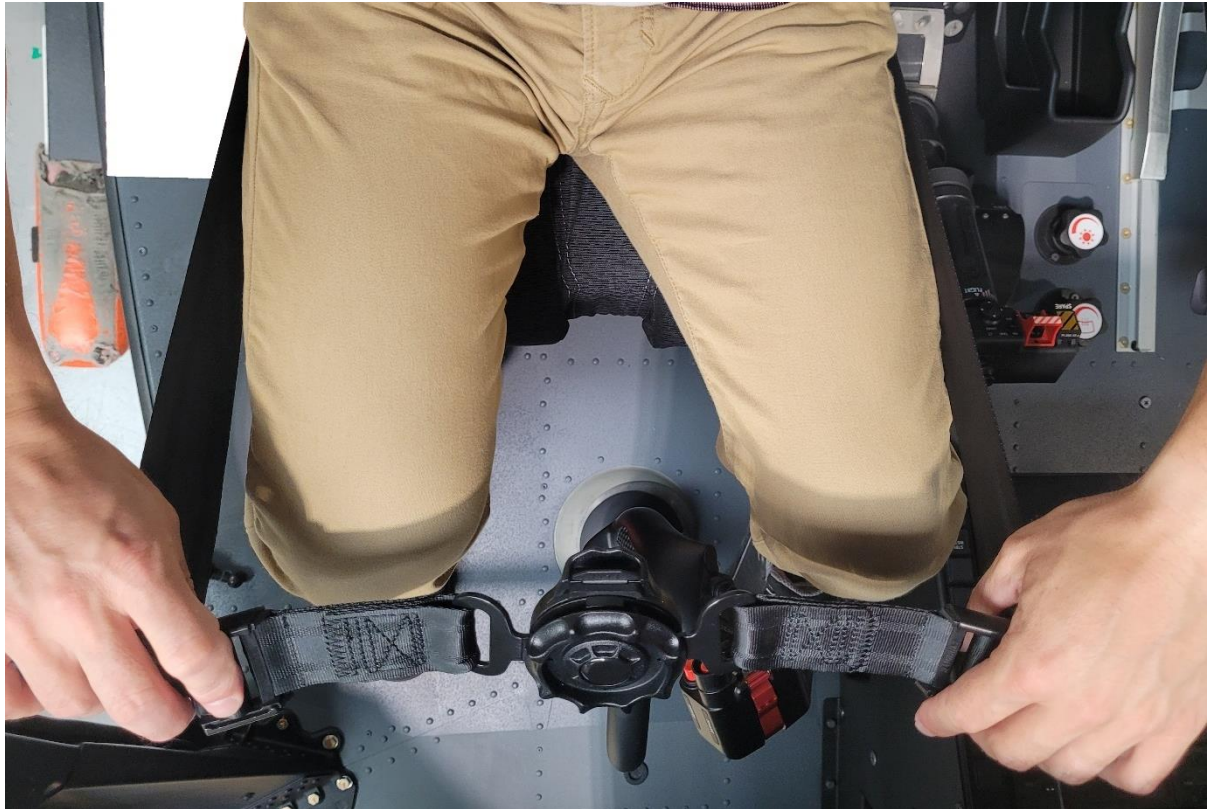
PHOTO 5 - The lap straps are long enough to be passed over the knees, meaning the legs can be released once the straps are placed on the floor of the aircraft. The seat occupant can easily evacuate the aircraft if necessary.
