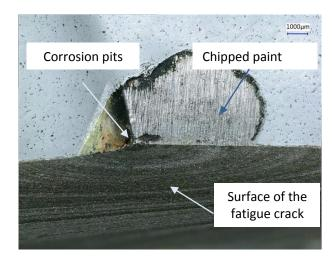
Any local damage associated with the lack of paint or protection can lead to corrosion over time. Corrosion pits locally modify the level of stress applied to the parts, which can end up in a fatigue crack initiation on the parts that are heavily stressed, such as the critical parts (rotor components, MGB suspension, etc.).
