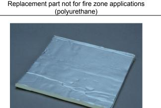
Pending the final investigation results, Airbus Helicopters would like to remind customers that the engine compartment is a designated fire zone and must resist and contain potential fire in accordance with type certification requirements. Therefore:
