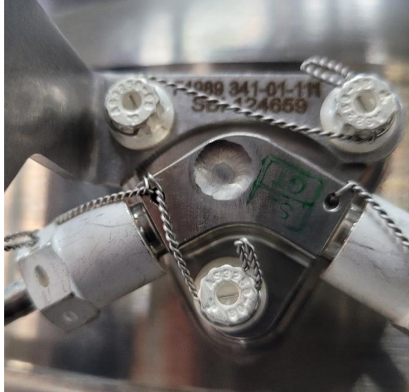
Figure 68: Locking of the screws attaching the ignition and main burners if the APU is in post-modification SB 342-49-048 configuration
