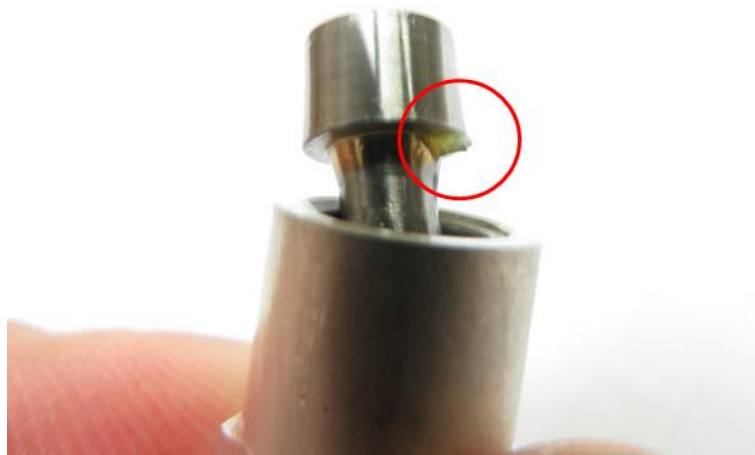
Figure 5: Location where application of a small amount of grease is required
