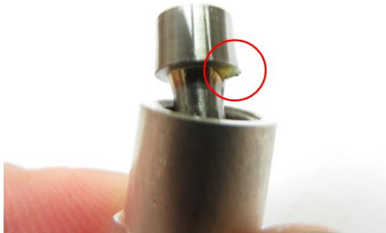
Figure 9: Location where application of a small amount of grease is required
