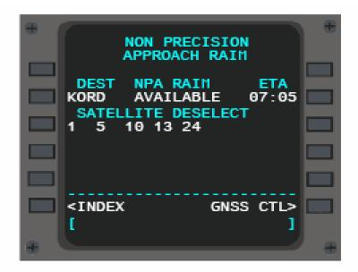
This function is only required when conducting a GNSS based approach outside of SBAS coverage or when SBAS is not available (check NOTAMs). Verification of Non Precision Approach RAIM availability is not required when conducting SBAS based approaches.
