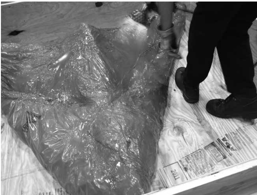
Forming a Wrap Around the Propeller Figure 3-4
