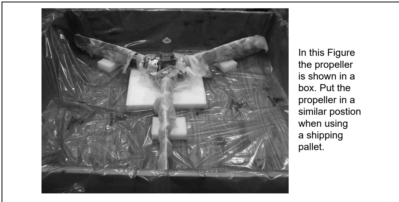
Putting the Propeller on the Foam Blocks Figure 3-2
