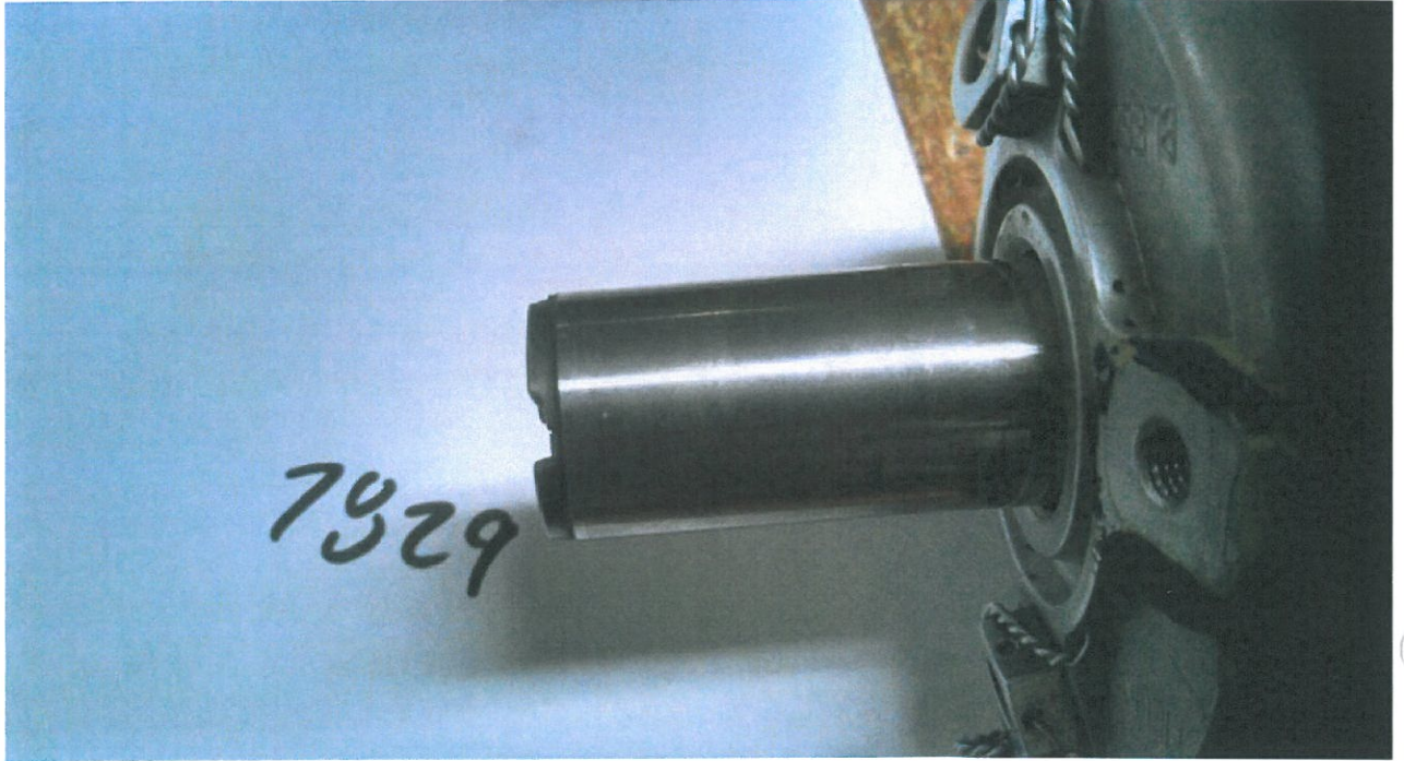
Sample of damage on piston slot
