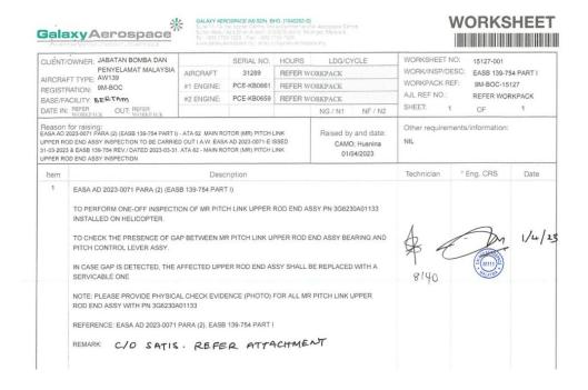
SB 139-754 Rev. / - Inspection Report 1/4/23 Date S/N FH Upper Rod End Assy P/N 3G6230A01133 MCR 08054 140:51 Installed on Helicopter Stock item D Installed on Pitch Link Assy S/N FH P/N 3G6230A01033 S/N (if applicable) 1407 3776:26 31289 Dimension "X" measurement N/A Notes: GAP NOT FOUND .
