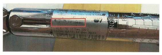
Tool ID No. CTE/30 torque wrench was sampled and found calibration sticker pasted on the tool was CTE/177.
