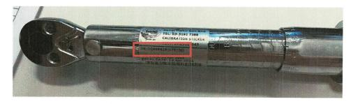
Tool ID No. CTE/177 (60640) torque wrench was sampled and found calibration sticker pasted on the tool was for CTE/30.
