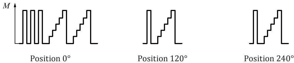
Figure C.2 — Examples of preloading and sequences for torque measurement devices with hexagon drive (minimum of four steps)
