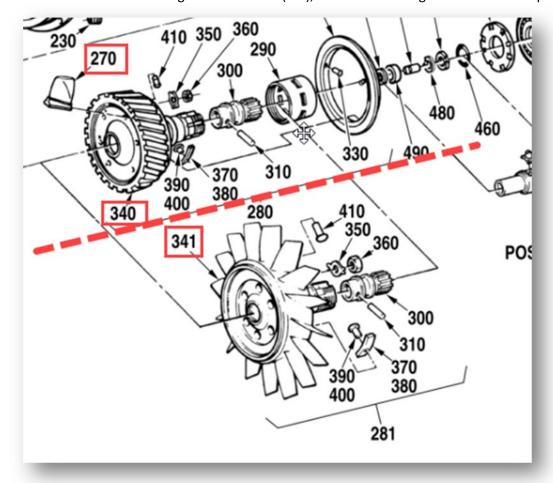
PK0985 LLP log shows PN 3041271 installed which is listed as item 341G in the IPC and has a an LCF limit of 15000 cycles.
