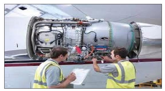
The approved steps of a maintenance procedure must be signed off by the LAE/technician doing the work as it is performed. Continuing a job that has been started by someone else should only occur after a face-to-face meeting of LAE/technicians. The applicable paperwork should be reviewed, the completed work discussed, and attention for the next step should be drawn. Absence of either a written or oral turnover serves as warning that an error could occur.
