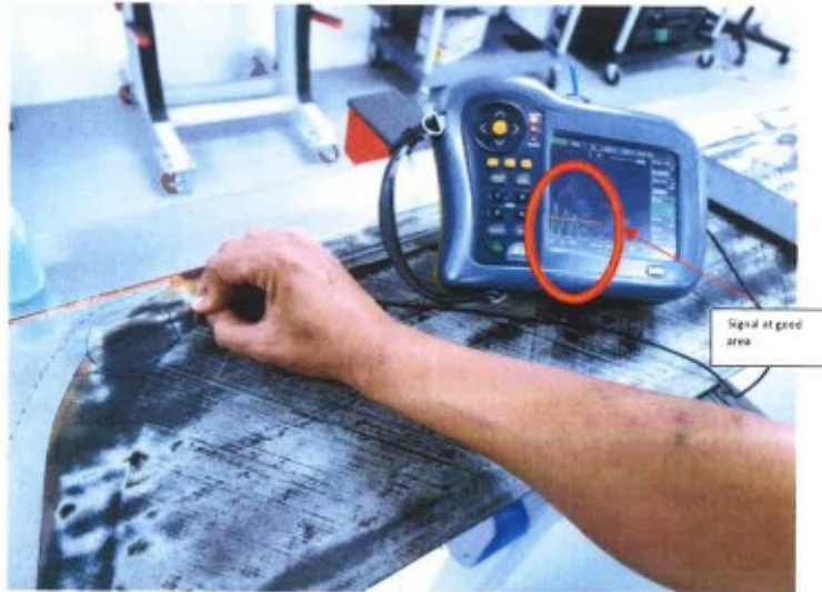
Tested signal at good area figure 2
