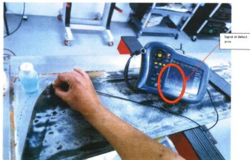
Figure 3 show drop in signal indicate delamination occur,
