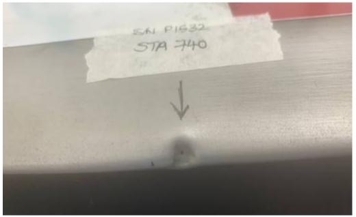
With reference to the A109S IETP DM 3C-A-64-11-01-00A-280A-C Step 10.2, sharp dents on the erosion shield are not permitted. We plan to trim and remove the marked area of the erosion shield as shown below to inspect whether the spar has been damaged as we believe that the blade can be sent back to Italy for an erosion shield replacement if the spar has not been damaged. Please advise if you have information to the contrary which would mean that our time is not wasted.
