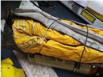
**P1** Aft float bag assembly received opened and sign of dirt's and water contamination
