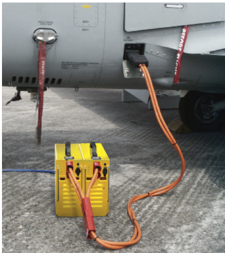
2 x PS100 in parallel: delivering up to 200 amps
