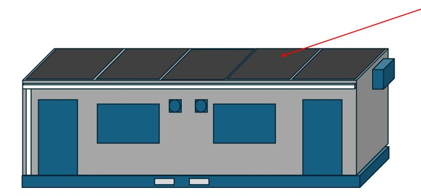
INSTALLING 2 MM 4' X 8 ' MILD STEEL SHEET WELDED TOGETHER TO UPPER CABIN FRAME
