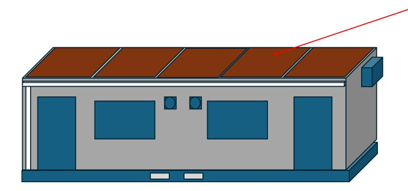
REMOVE INNER SHELL (9 MM WATERPROOF PLYWOOD) OF CABIN ROOF THAT BADLY INFECTED BY TERMITES
