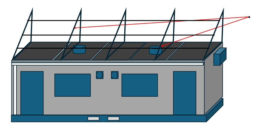
REINSTALL FRAME STRUCTURE TO ALLOW INSTALLATION OF ADDITIONAL ROOF (ADDITIONAL PROTECTION)
