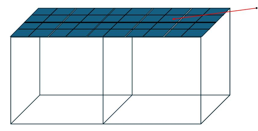
REMOVE DAMAGED AND INFECTED INNER CEILING WITH 6 MM CEMENT BOARD SCREWED TO UPPER FRAME
