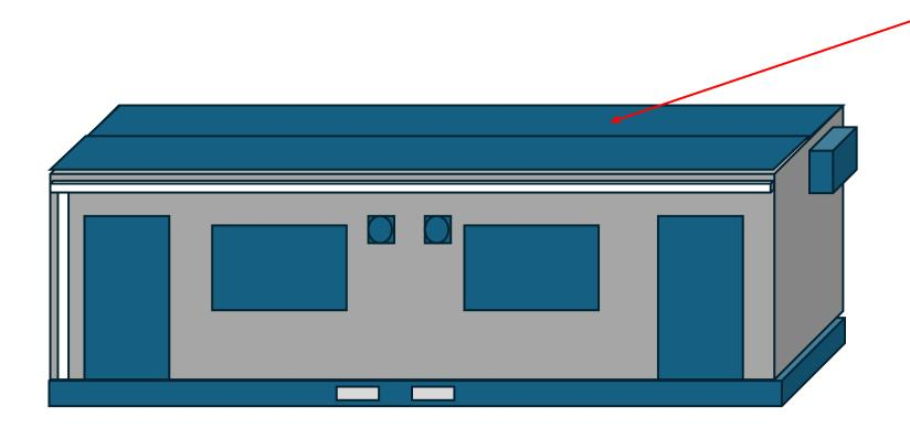
REMOVE OUTER SHELL (GALVANIZE STEEL SHEET) OF CABIN ROOF GLUED AND RIVETTED TO UPPER CABIN FRAME
