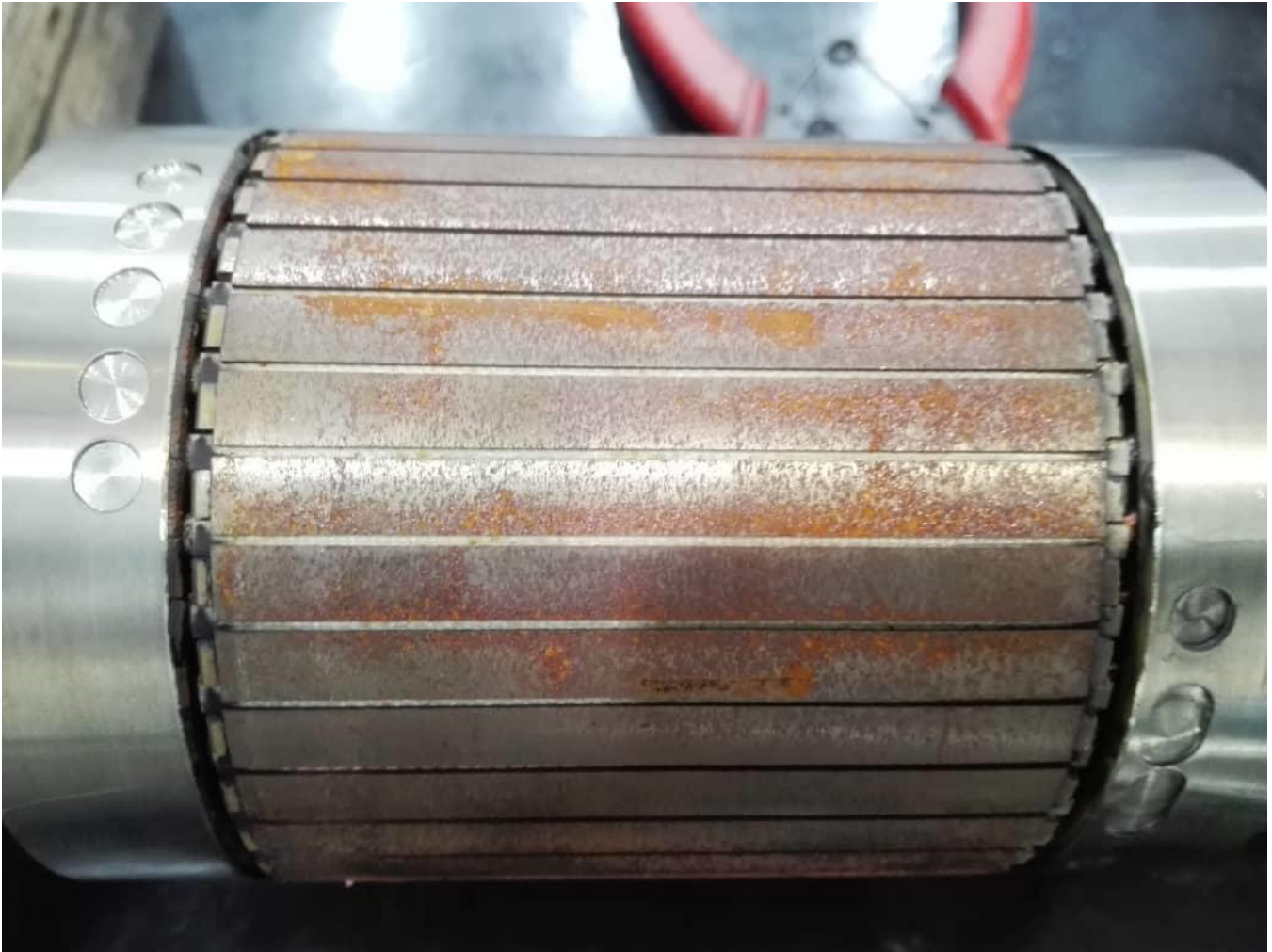
Photo (1) : Armature assembly – sign of water mark and rust at the bottom half
