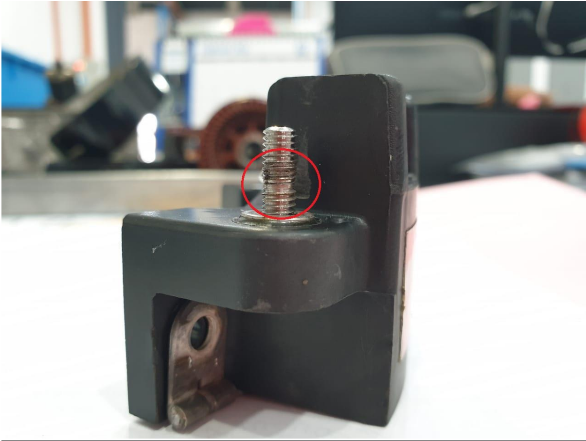
Photo 1 – Terminal block thread stripped.
