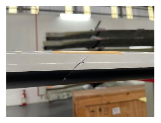
o Swept tip erosion shield found edge void
